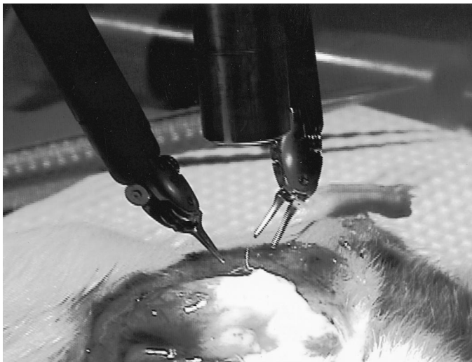
FIG. 3. Animal was transferred to surgical robot field for microsurgical anastomosis.
