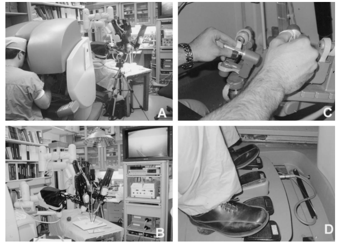
FIG. 1. Initial experience with robot involved familiarizing operating surgeon with robot design and setup in laboratory (A) and some robotic exercises involved placing sutures (B) on practice card with robotic hand and foot coordination (C and D).
